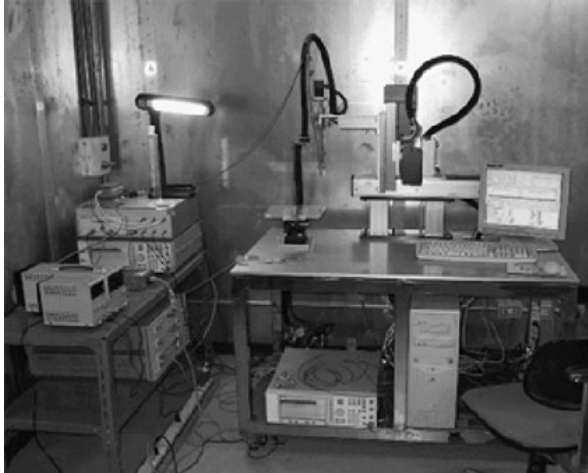
Figure 10. The photograph of the adjacent field distributions measurement system.
