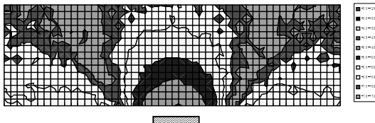
Figure 6. Electric and magnetic field distributions above the microstrip line at 1.5 GHz (parallel to the line)
